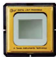
Digital image generation instead of an analog GOBO
